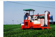
Riding-type plucking machine
