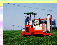
Riding-type plucking machine
